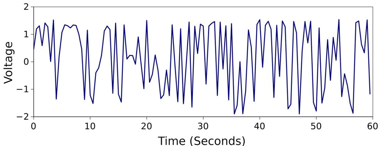
Fig. 6. Voltage corresponding to the sensed magnetic field. The actual voltage signal is unipolar. In this representation, the voltage is subtracted from the mean value of the entire time series to show a bipolar response.
