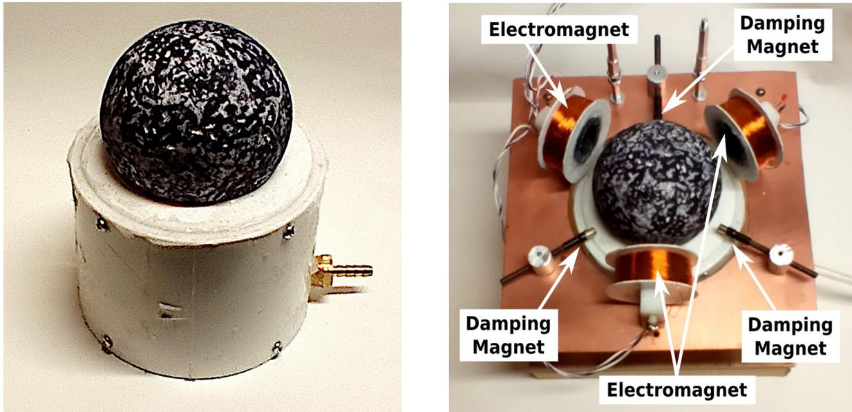
Fig. 2. Left, the finished sphere seated in its air bearing. Right, placement of the electromagnets. Also shown are the three damping magnets described in the text. Air was supplied by a Porter Cable Model C2002 Portable Electric Pancake Air Compressor with an airflow of about 3 cubic feet per minute.
