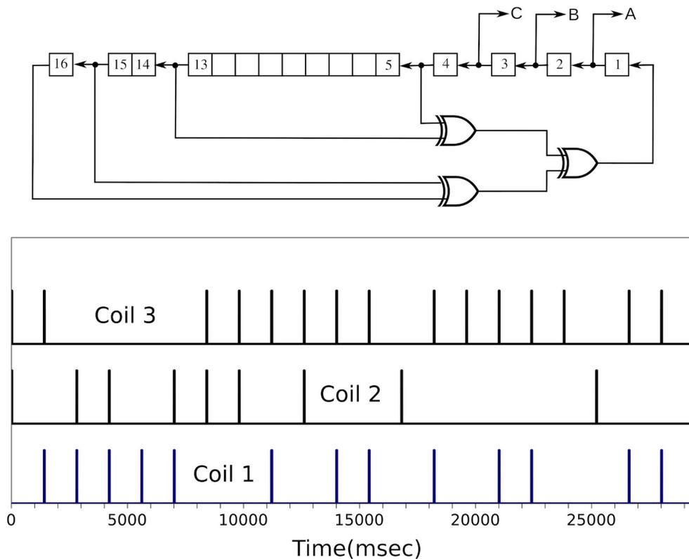
Fig. 3. Top, the linear feedback shift register used for generation of pseudorandom pulse excitation of the electromagnets. Bottom, a portion of the excitation sequence.
