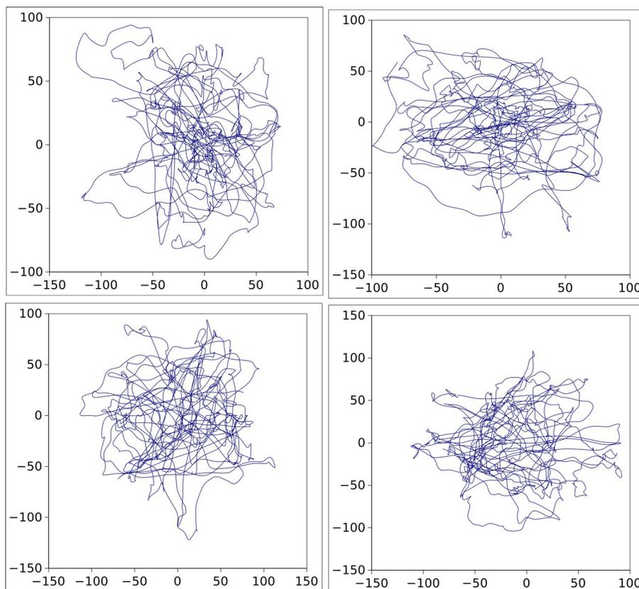
Fig. 5. Sphere motion as detected by the optical sensor of an optical mouse. The sensor gives incremental motion in "x" and "y" directions in a range of  $\pm 127$ .
