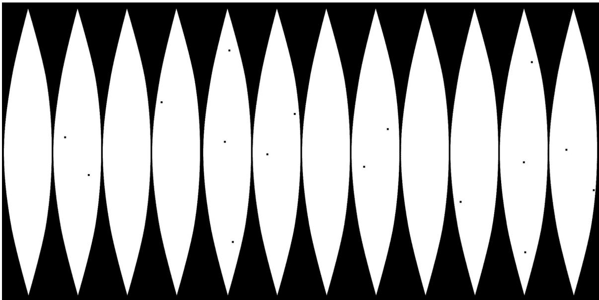
Fig. 1 . Gore pattern used to facilitate drilling of holes for magnet placement in the sphere. Each hole is paired with another on the opposite side of the sphere.
